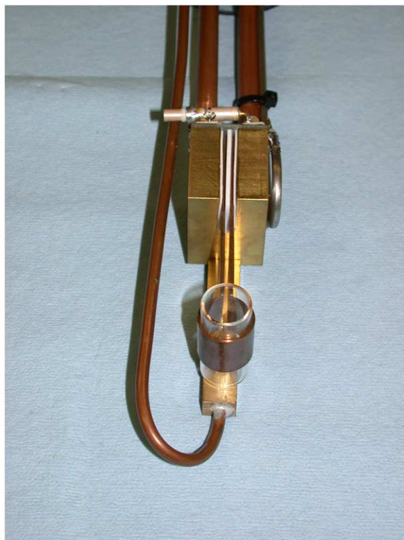
Fig. 2. Photographs of probe: (A) showing end view with gas inlet and loop-gap resonator enclosing quartz tube. (B) The probe mounted in 75 mm diameter poly-carbonate tube. The fume hood above the flame and part of the thin copper sheet RF screen can be seen. During operation a further RF screen is present which reduces RF coupling to the gradients as well as assisting in distributing any heat away from the hood area.
